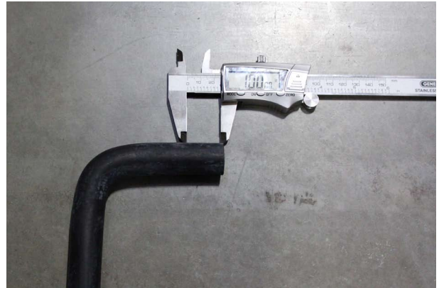
Fig. 5-f: Remove 1" Of Hose
