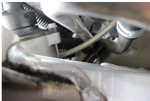
Fig. 11-b: Route Oil Feed Line
