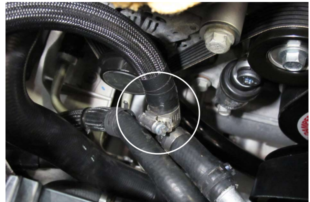
Fig. 5-v: Install 3ft Length Of 5/8" Coolant Hose & Secure
