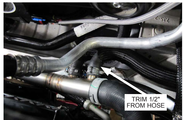
Fig. 5-e: Trim 1/2" From Suppl. Radiator Hose (Closest to driver side wheel well.)
