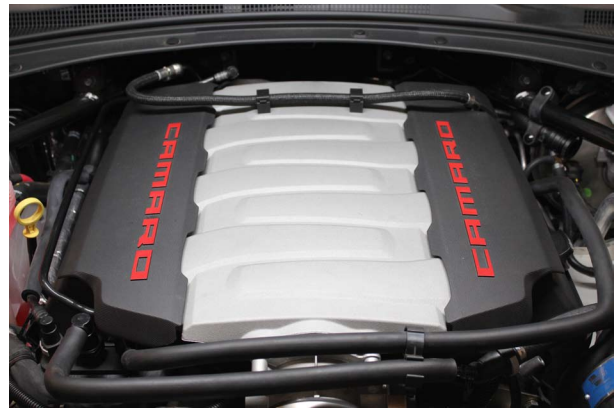
Fig. 9-a: Remove "CAMARO" Engine Covers
