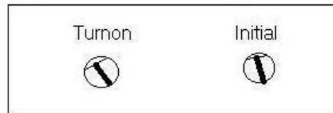
This is typical factory preset for a GM 2 bar application. IE Corvette 2.7 volts DC
