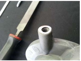
■ The factory C6 Slave Cylinder has some casting marks that need to be filed down. Using a simple hand file, smooth down the bleeder boss to create a smooth mating surface for the sealing washer. Make sure to clean out any metal shavings out of the bleeder boss.
