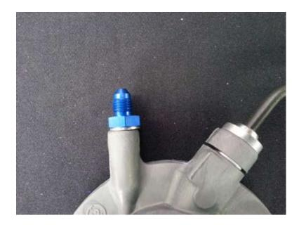
■ Next, install the supplied AN fitting to the Slave Cylinder using the supplied O-ring washer, as shown above.
