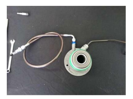
■ Your Slave Cylinder is now ready for assembly to your transmission. Once installed in the car, make sure you route the bleeder hose away from any heat or moving parts to a location under the hood that is easy to access for bleeding. If you have any questions contact East Coast Supercharging.
