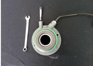
• Using 9mm wrench, remove the factory bleeder from your GM C6 Slave Cylinder, as shown above.
