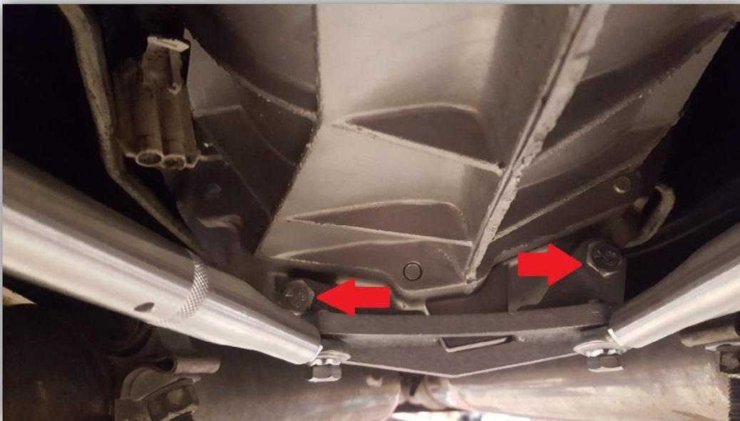
Strut bars assembly and install:
