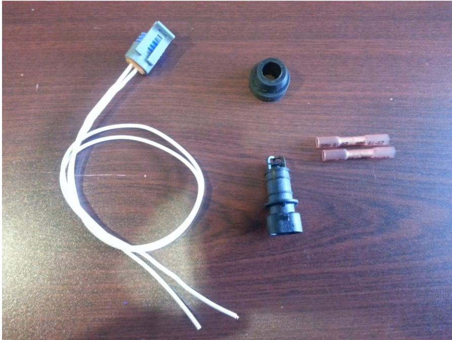
IAT Breakout: Both wires on the IAT sensor harness are reverse polarity. On the MAF sensor locate and cut the White/Light-Blue wire in pin #1 on the MAF sensor and the Black/Violet wire in pin #3 on the MAF and connect those to the wires from the IAT sensor harness using the supplied connectors.
