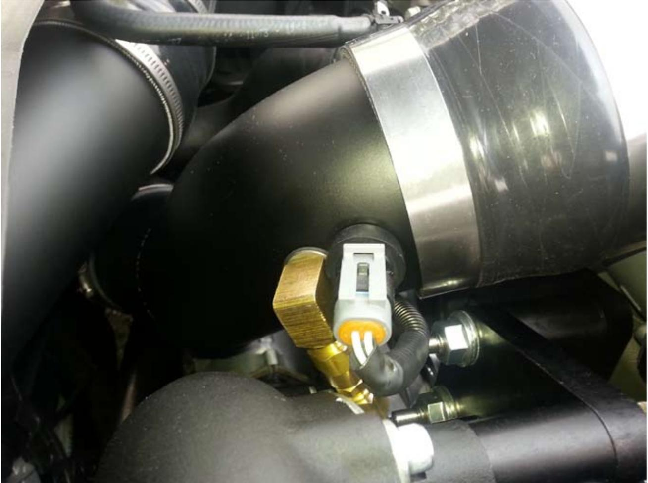
To do so, first is mark where the hole will be before removing the charge pipe. Next is drill hole into charge tube 3/8 diameter and clean up the hole from debris. The nozzle has two washers included. If nozzles are going into aluminum, the rubber washers help seal the nozzle.
