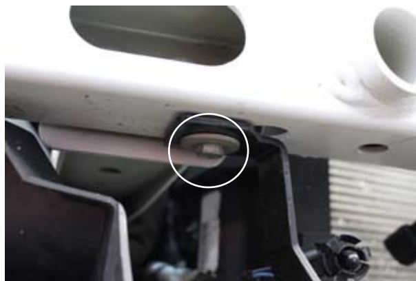
Fig. 1-n: Remove Trans Cooler Mount Screws
