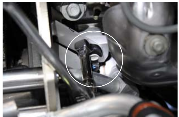
Fig. 4-l: Re-tighten A/C Mount Screw
