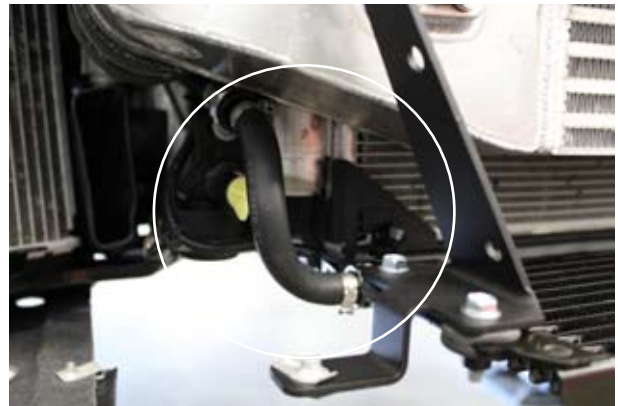
Fig. 2-h: Install Provided Trans. Cooler Line
