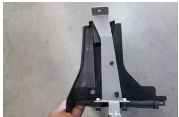
Fig. 2-c: Temporarily Mount New Trans. Cooler Bracket
