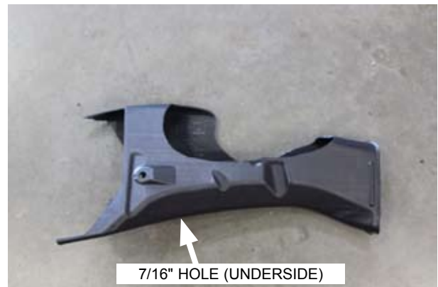
Fig. 6-b: Modified Brake Cooling Duct (Inner Section)
