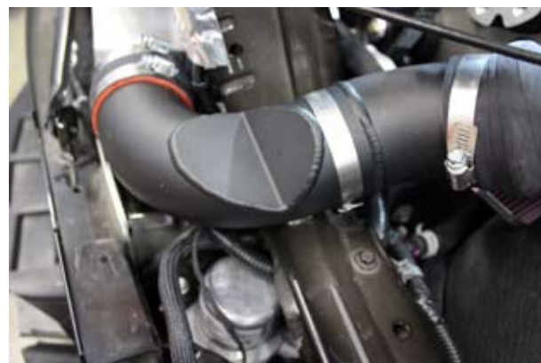
Fig. 5-c: Install Discharge Tube "B" As Shown
