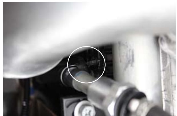
Fig. 2-f: Detach Trans. Cooler Line From Radiator
