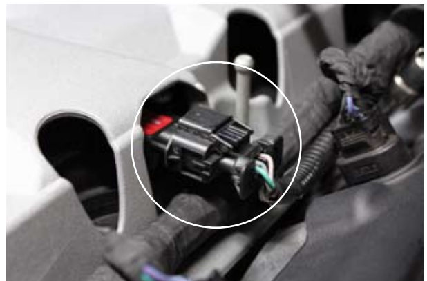
Fig. 7-c: Unplug MAP Sensor Connector
