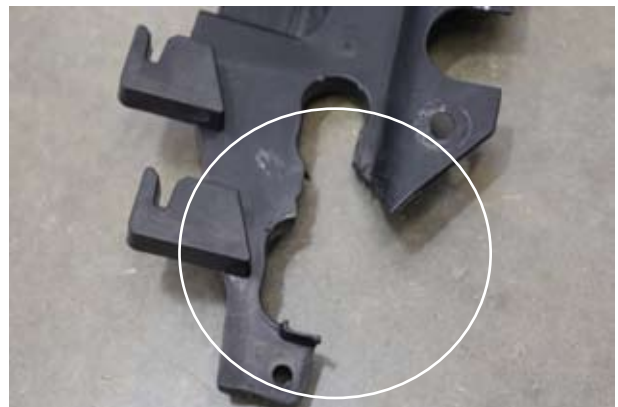
Fig. 1-x: Cut Radiator Shroud As Shown
