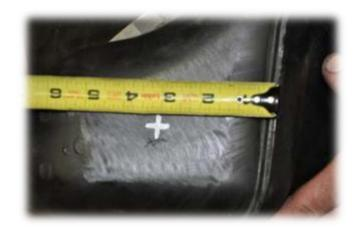
With a 90 degree drill, or a long drill extention, Use the supplied 1 ¾ hole saw, drill tank as shown being sure to de burr tank and clean any residual debris from tank afterwards.
