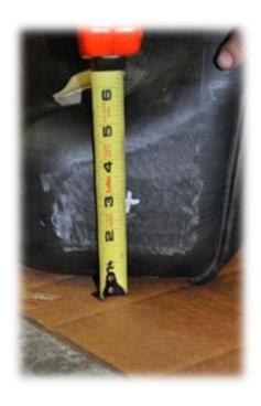
Approximately 3 inches from seam and 2 ¾ inches from bottom of tank make a mark where you will be drilling for the ECS in tank auxiliary fuel pick up assembly.
