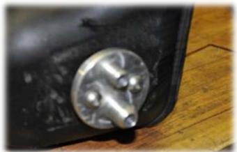
Install second allen bolt (with o-ring) and snug down. Torque bots down to 12 ft/pounds.
