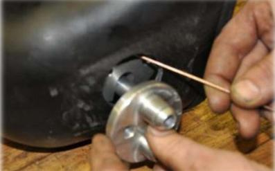
Slide backer plate over fuel pick up tube
