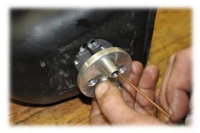
Reinsert wire tool into backer plate through return opening or one of the screw holes to support backer plate holding it against the back of the tank.
