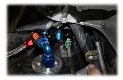
The Fuel Line adapter will snap in place between the factory fuel pump outlet and the factory fuel feed line as shown below.
