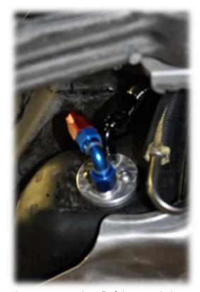
Take approximately 14" of the Provided 6AN Braided Fuel Line and Install a 45deg fitting on each end. This line will run from the outlet side of the pump to factory fuel line. On the fuel line side, install the provided male/male 6an union, and the provided fuel line adapter as shown.
